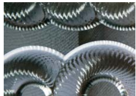
Fräsbild Hydrodehnspannfutter Milling image of hydraulic chuck
