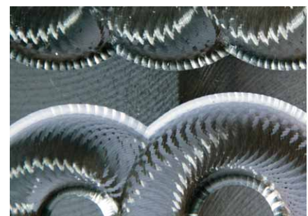
Fräsbild Hydrodehnspannfutter Milling image of hydraulic chuck
